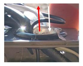
Pull the pre-existing antenna out through the silicone covered hole at the top at the top of the PC Board housing. (\*\*RED Arrow\*\*)
