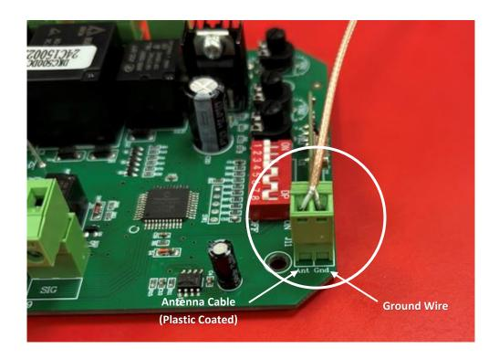
To install a GTR129 External Antenna, you must locate the Antenna terminals on your relevant Richmond Sliding Gate Motor's PC Board. The two terminals will be labelled "Ant" & "Gnd".
