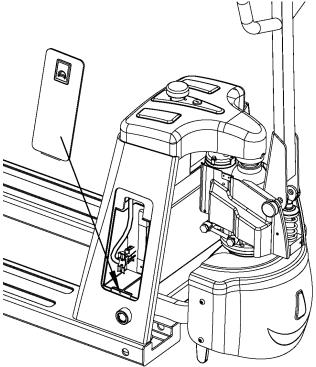
Remove the cable harness, push the battery fastening buckle to the left, pull the battery handle outward, and take out the battery. Otherwise, put the battery into the battery.
