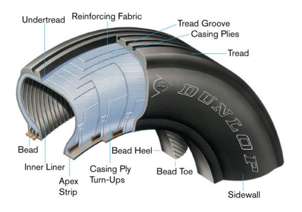
Tyres with a higher ply rating will take high air pressures and in turn can carry greater loads.
