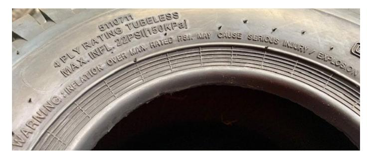
There may be two PSI ratings shown on the tyre – 22psi and a warning pressure - Never exceed 35psi to seat the beads.
